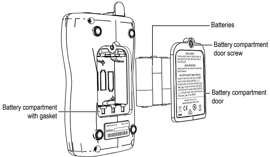
Figure 2-2 Opening the battery compartment
