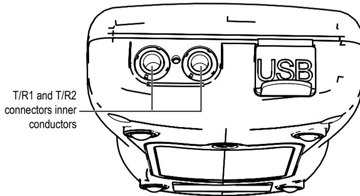
**Figure i-2 Risk of electrical shock on T/R connectors inner conductors**
