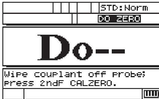
**Figure 4-1 Transducer zero compensation**
