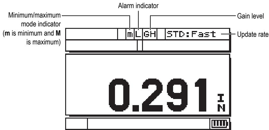
Figure 3-2 Other elements of the measurement screen
