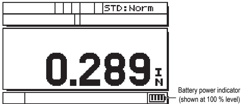
Figure 2-1 The power indicator when using batteries
