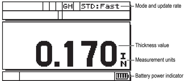
Figure 3-1 The measurement screen
