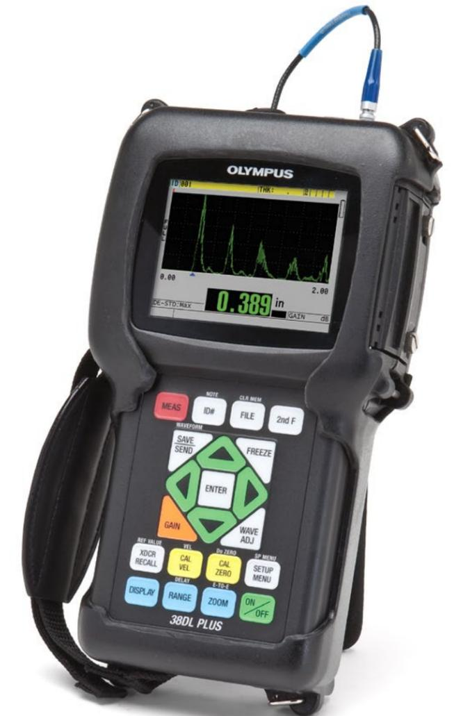
38DL PLUS thickness gage with standard protective rubber boot
