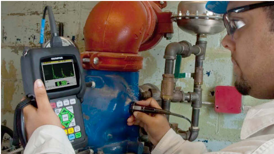
Figure 1-1 Measuring thicknesses with the 38DL PLUS
