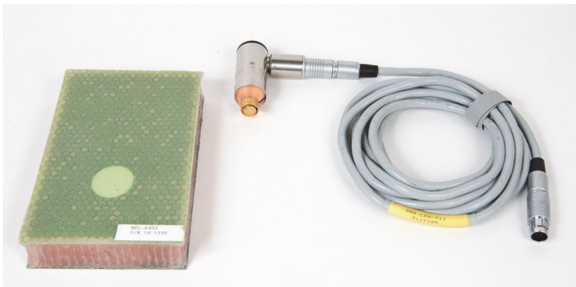
Figure 6-29 Materials — repaired areas (potting) using MIA technique
