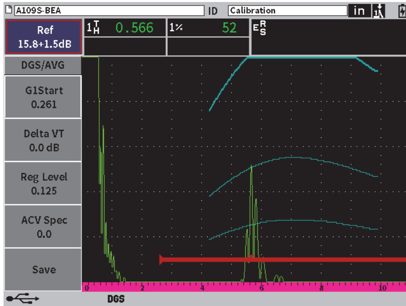
Figure 11-23 Gain curve adjusted DGS
