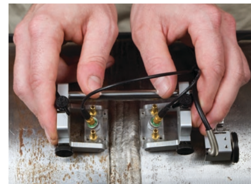
The HST-X04™ TOFD manual scanner offers an efficient, low-cost weld inspection solution.
