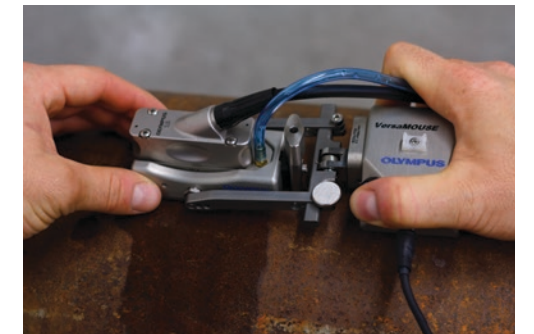
VersaMOUSE and RexoFORM scanners for corrosion inspection.
