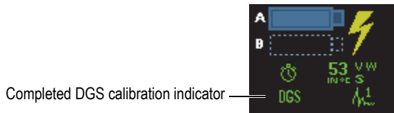
Figure 5-24 Completed DGS calibration status indicator
