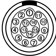
Figure 7-2 The scanner interface LEMO connector (pin side)
