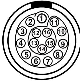
**Figure 7-3 The scanner interface adaptor LEMO connector (weld side)**
