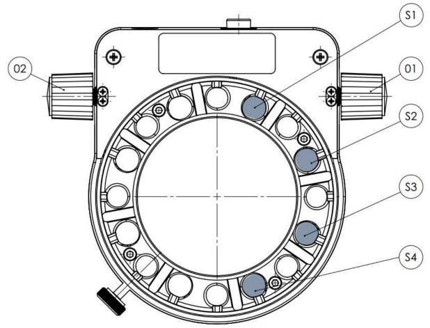
There are 4 setting points for which one LED (S1-S4) is available for each. By turning the encoder (1), you can control the desired setting point. Pressing the same encoder (1) changes the value of this setting. The set value is indicated by the flashing or lighting of the respective LED.
