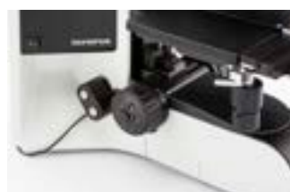
Hand switch for motorized nosepiece rotation
