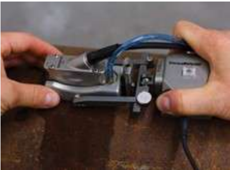
VersaMOUSE and RexoFORM scanners for corrosion inspection.
