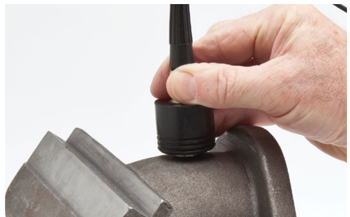
Many cast metal parts or sound-attenuating materials can be measured with the High Penetration software option.
